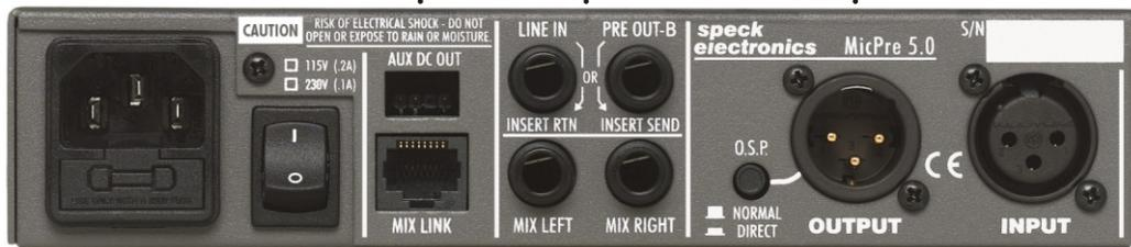
The **Mix Link** connector allows the mix section of the MP5.0 to be combined with any number of MP5.0's to form a fully integrated mix section.
